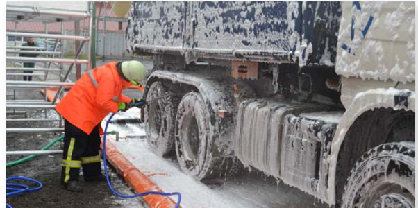
Due to the flexible edge limitation, a smooth entry into the tub without loss of disinfectant is possible.
